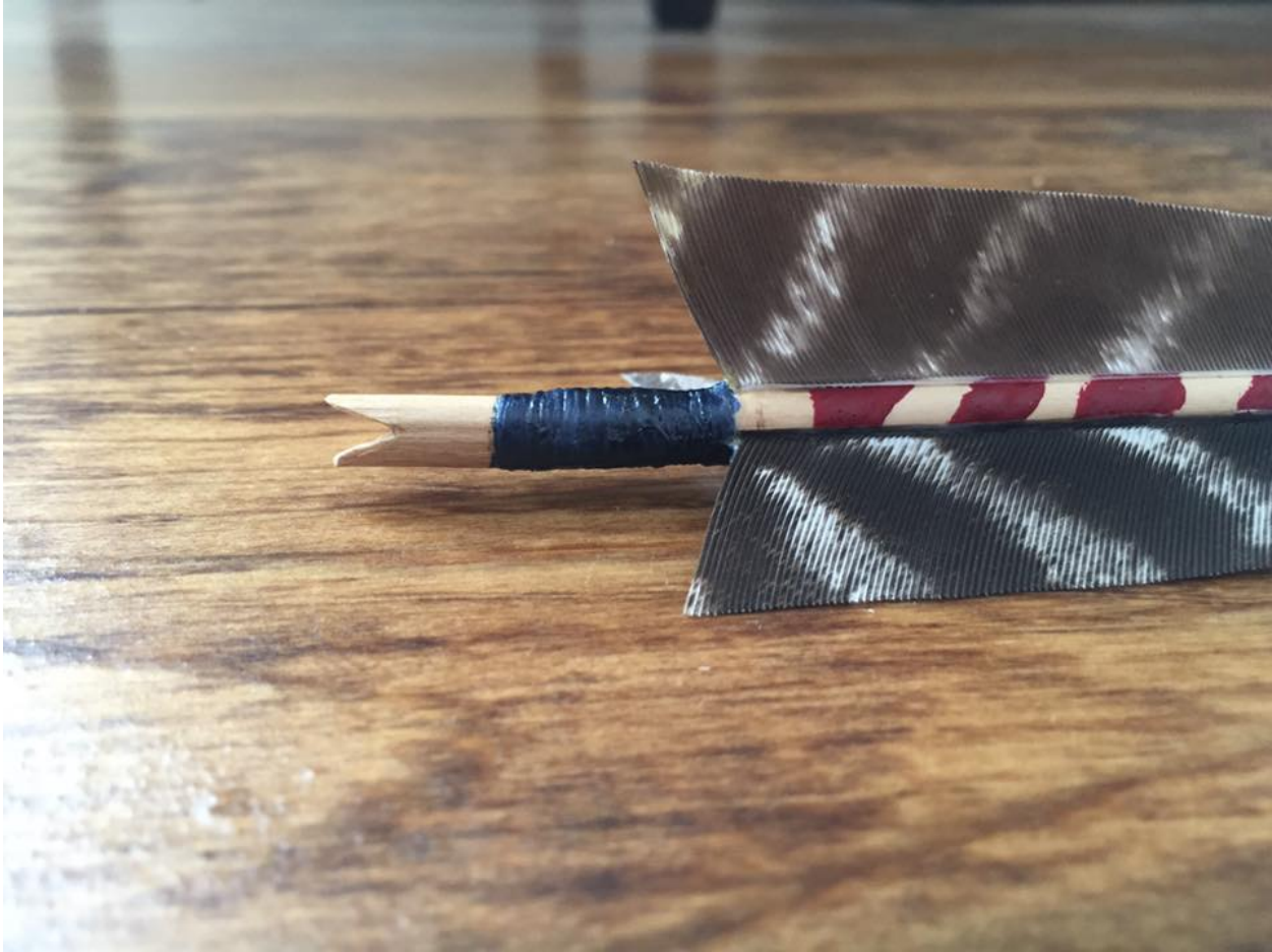
Figure 11: Nock end of the same arrow, sinew binding and painting.
